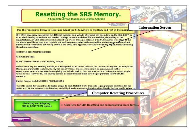
Many times it is necessary to disconnect or disable other modules or computers to repair an SRS problem. For the most part, there will also be a need to remove the vehicle's battery whenever dealing with any SRS dangerous component, such as an airbag. This presents a problem, since most modules will loose the adaptive memory whenever the battery gets disconnected.
