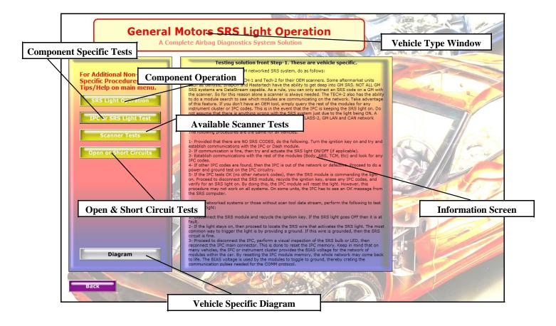
This is Step 2 at its best. This screen is just one of the many component tests and procedures intended as "Vehicle Specific" program areas. Every time the technician goes to Step 1, the vehicle make is stored in memory. So that when he/she enters step 2, the software remembers the manufacturer and provides only the relevant information far that type of SRS system.
