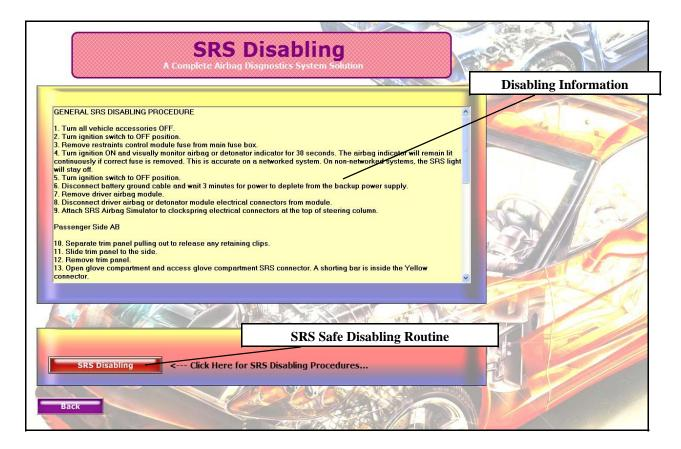
This screen provides the technician with information destine to disable the SRS airbag system. Often time this routine is ignored by the techs, by it is an integral part of the SRS repair process.
