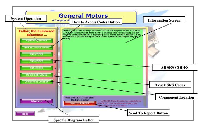
**VEHICLE SPECIFIC SCREEN:** Within this screen you have the ability to start the SRS diagnostics process with vehicle specific SRS codes, electrical testing procedures, how to access SRS codes, and component locations. Then at the bottom you have a button that (RED) allows you to send the information to a report found on the main menu.
